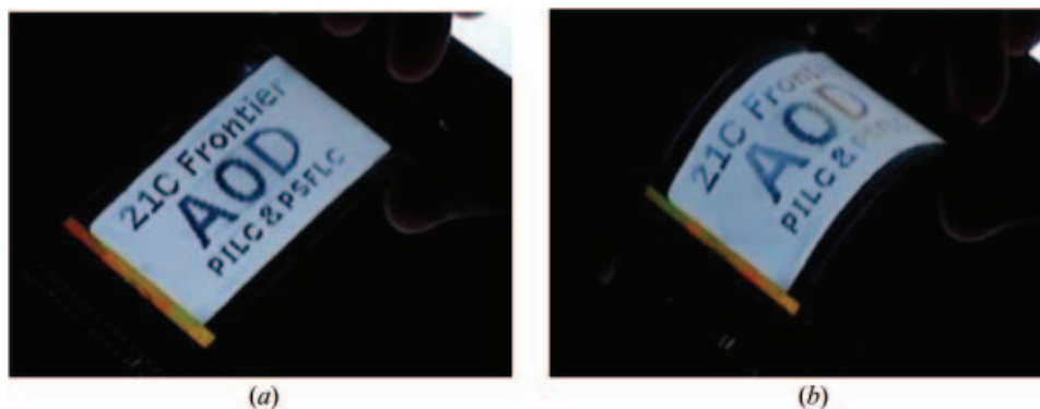
Figure 9. (a) Photograph of the memory state at 0V, (b) curved shape like a paper for the Co(16)-LCP/E7 (30/70 wt%).
